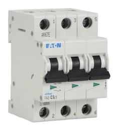
Eaton miniature supplementary protector, 5A, 480Y / 277 VAC / 96 VDC, 3-pole, C curve, thermal magnetic, 10kA @ 480Y/277 VAC interrupting rating, 35mm DIN rail mount.
