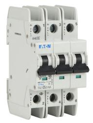
Eaton miniature circuit breaker, current-limiting, 5A, 480Y / 277 VAC / 96 VDC, 3-pole, C curve, thermal magnetic, 10kA @ 480Y/277 VAC interrupting rating, 35mm DIN rail mount.
