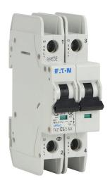
Eaton miniature circuit breaker, current-limiting, 5A, 480Y / 277 VAC / 96 VDC, 2-pole, C curve, thermal magnetic, 10kA @ 480Y/277 VAC interrupting rating, 35mm DIN rail mount.
