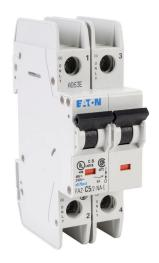
Eaton miniature circuit breaker, current-limiting, 5A, 240 VAC / 96 VDC, 2-pole, C curve, thermal magnetic, 10kA @ 240 VAC interrupting rating, 35mm DIN rail mount.
