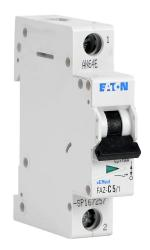
Eaton miniature supplementary protector, 5A, 277 VAC / 48 VDC, 1-pole, C curve, thermal magnetic, 10kA @ 277 VAC interrupting rating, 35mm DIN rail mount.
