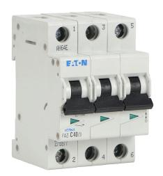
Eaton miniature supplementary protector, 40A, 480Y / 277 VAC / 96 VDC, 3-pole, C curve, thermal magnetic, 5kA @ 480Y/277 VAC interrupting rating, 35mm DIN rail mount.
