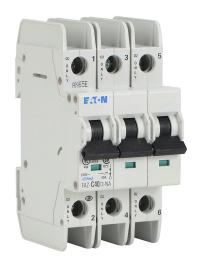
Eaton miniature circuit breaker, current-limiting, 40A, 240 VAC / 48 VDC, 3-pole, C curve, thermal magnetic, 10kA @ 240 VAC interrupting rating, 35mm DIN rail mount.
