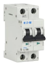
Eaton miniature supplementary protector, 40A, 480Y / 277 VAC / 96 VDC, 2-pole, C curve, thermal magnetic, 5kA @ 480Y/277 VAC interrupting rating, 35mm DIN rail mount.
