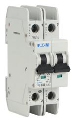
Eaton miniature circuit breaker, current-limiting, 40A, 240 VAC / 48 VDC, 2-pole, C curve, thermal magnetic, 10kA @ 240 VAC interrupting rating, 35mm DIN rail mount.
