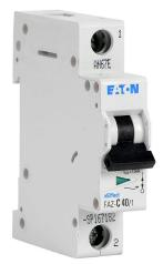
Eaton miniature supplementary protector, 40A, 277 VAC / 48 VDC, 1-pole, C curve, thermal magnetic, 5kA @ 277 VAC interrupting rating, 35mm DIN rail mount.
