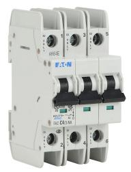
Eaton miniature circuit breaker, current-limiting, 4A, 480Y / 277 VAC / 96 VDC, 3-pole, C curve, thermal magnetic, 10kA @ 480Y/277 VAC interrupting rating, 35mm DIN rail mount.
