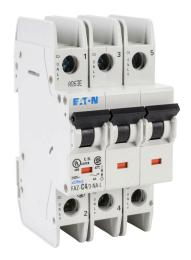
Eaton miniature circuit breaker, current-limiting, 4A, 240 VAC / 96 VDC, 3-pole, C curve, thermal magnetic, 10kA @ 240 VAC interrupting rating, 35mm DIN rail mount.
