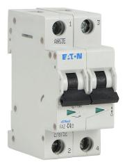
Eaton miniature supplementary protector, 4A, 480Y / 277 VAC / 96 VDC, 2-pole, C curve, thermal magnetic, 10kA @ 480Y/277 VAC interrupting rating, 35mm DIN rail mount.
