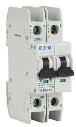
Eaton miniature circuit breaker, current-limiting, 4A, 480Y / 277 VAC / 96 VDC, 2-pole, C curve, thermal magnetic, 10kA @ 480Y/277 VAC interrupting rating, 35mm DIN rail mount.
