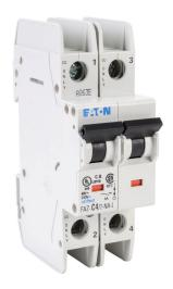
Eaton miniature circuit breaker, current-limiting, 4A, 240 VAC / 96 VDC, 2-pole, C curve, thermal magnetic, 10kA @ 240 VAC interrupting rating, 35mm DIN rail mount.
