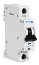
Eaton miniature supplementary protector, 4A, 277 VAC / 48 VDC, 1-pole, C curve, thermal magnetic, 10kA @ 277 VAC interrupting rating, 35mm DIN rail mount.
