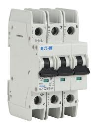
Eaton miniature circuit breaker, current-limiting, 35A, 240 VAC / 48 VDC, 3-pole, C curve, thermal magnetic, 10kA @ 240 VAC interrupting rating, 35mm DIN rail mount.
