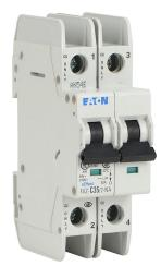
Eaton miniature circuit breaker, current-limiting, 35A, 240 VAC / 48 VDC, 2-pole, C curve, thermal magnetic, 10kA @ 240 VAC interrupting rating, 35mm DIN rail mount.
