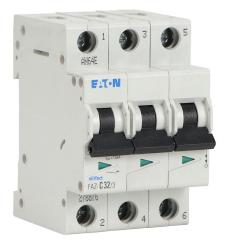
Eaton miniature supplementary protector, 32A, 480Y / 277 VAC / 96 VDC, 3-pole, C curve, thermal magnetic, 10kA @ 480Y/277 VAC interrupting rating, 35mm DIN rail mount.
