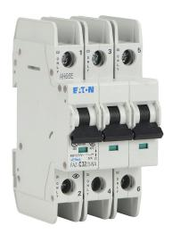
Eaton miniature circuit breaker, current-limiting, 32A, 480Y / 277 VAC / 96 VDC, 3-pole, C curve, thermal magnetic, 10kA @ 480Y/277 VAC interrupting rating, 35mm DIN rail mount.
