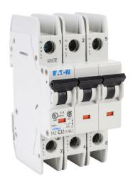
Eaton miniature circuit breaker, current-limiting, 32A, 240 VAC / 96 VDC, 3-pole, C curve, thermal magnetic, 10kA @ 240 VAC interrupting rating, 35mm DIN rail mount.
