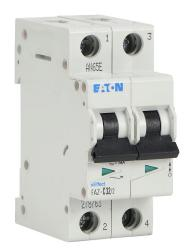
Eaton miniature supplementary protector, 32A, 480Y / 277 VAC / 96 VDC, 2-pole, C curve, thermal magnetic, 10kA @ 480Y/277 VAC interrupting rating, 35mm DIN rail mount.
