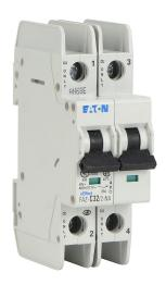
Eaton miniature circuit breaker, current-limiting, 32A, 480Y / 277 VAC / 96 VDC, 2-pole, C curve, thermal magnetic, 10kA @ 480Y/277 VAC interrupting rating, 35mm DIN rail mount.
