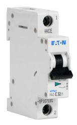
Eaton miniature supplementary protector, 32A, 277 VAC / 48 VDC, 1-pole, C curve, thermal magnetic, 10kA @ 277 VAC interrupting rating, 35mm DIN rail mount.
