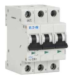
Eaton miniature supplementary protector, 30A, 480Y / 277 VAC / 96 VDC, 3-pole, C curve, thermal magnetic, 10kA @ 480Y/277 VAC interrupting rating, 35mm DIN rail mount.
