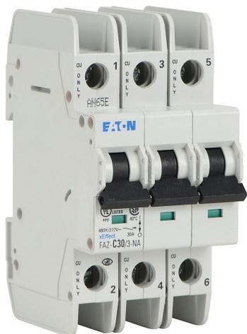
Eaton miniature circuit breaker, current-limiting, 30A, 480Y / 277 VAC / 96 VDC, 3-pole, C curve, thermal magnetic, 10kA @ 480Y/277 VAC interrupting rating, 35mm DIN rail mount.
