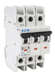
Eaton miniature circuit breaker, current-limiting, 30A, 240 VAC / 96 VDC, 3-pole, C curve, thermal magnetic, 10kA @ 240 VAC interrupting rating, 35mm DIN rail mount.
