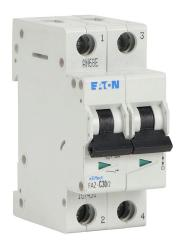
Eaton miniature supplementary protector, 30A, 480Y / 277 VAC / 96 VDC, 2-pole, C curve, thermal magnetic, 10kA @ 480Y/277 VAC interrupting rating, 35mm DIN rail mount.
