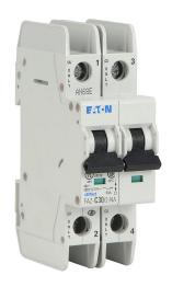
Eaton miniature circuit breaker, current-limiting, 30A, 480Y / 277 VAC / 96 VDC, 2-pole, C curve, thermal magnetic, 10kA @ 480Y/277 VAC interrupting rating, 35mm DIN rail mount.
