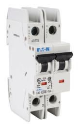
Eaton miniature circuit breaker, current-limiting, 30A, 240 VAC / 96 VDC, 2-pole, C curve, thermal magnetic, 10kA @ 240 VAC interrupting rating, 35mm DIN rail mount.
