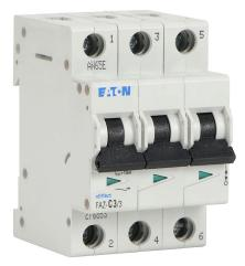
Eaton miniature supplementary protector, 3A, 480Y / 277 VAC / 96 VDC, 3-pole, C curve, thermal magnetic, 10kA @ 480Y/277 VAC interrupting rating, 35mm DIN rail mount.
