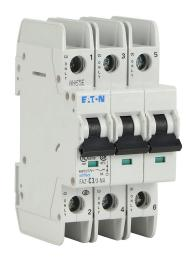
Eaton miniature circuit breaker, current-limiting, 3A, 480Y / 277 VAC / 96 VDC, 3-pole, C curve, thermal magnetic, 10kA @ 480Y/277 VAC interrupting rating, 35mm DIN rail mount.
