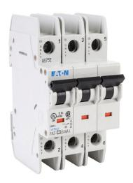
Eaton miniature circuit breaker, current-limiting, 3A, 240 VAC / 96 VDC, 3-pole, C curve, thermal magnetic, 10kA @ 240 VAC interrupting rating, 35mm DIN rail mount.
