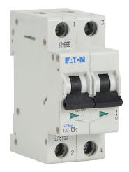
Eaton miniature supplementary protector, 3A, 480Y / 277 VAC / 96 VDC, 2-pole, C curve, thermal magnetic, 10kA @ 480Y/277 VAC interrupting rating, 35mm DIN rail mount.
