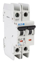
Eaton miniature circuit breaker, current-limiting, 3A, 240 VAC / 96 VDC, 2-pole, C curve, thermal magnetic, 10kA @ 240 VAC interrupting rating, 35mm DIN rail mount.
