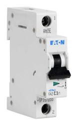
Eaton miniature supplementary protector, 3A, 277 VAC / 48 VDC, 1-pole, C curve, thermal magnetic, 10kA @ 277 VAC interrupting rating, 35mm DIN rail mount.
