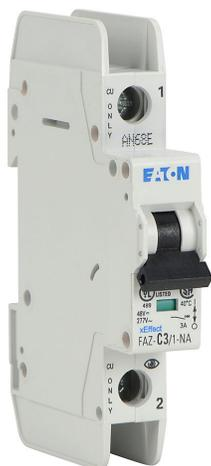
Eaton miniature circuit breaker, current-limiting, 3A, 277 VAC / 48 VDC, 1-pole, C curve, thermal magnetic, 10kA @ 277 VAC interrupting rating, 35mm DIN rail mount.
