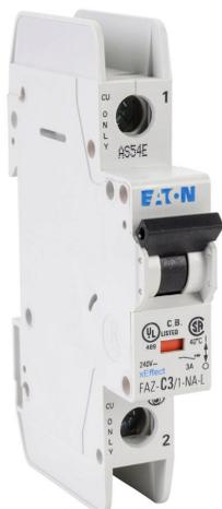
Eaton miniature circuit breaker, current-limiting, 3A, 240 VAC / 48 VDC, 1-pole, C curve, thermal magnetic, 10kA @ 240 VAC interrupting rating, 35mm DIN rail mount.
