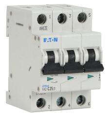
Eaton miniature supplementary protector, 25A, 480Y / 277 VAC / 96 VDC, 3-pole, C curve, thermal magnetic, 10kA @ 480Y/277 VAC interrupting rating, 35mm DIN rail mount.
