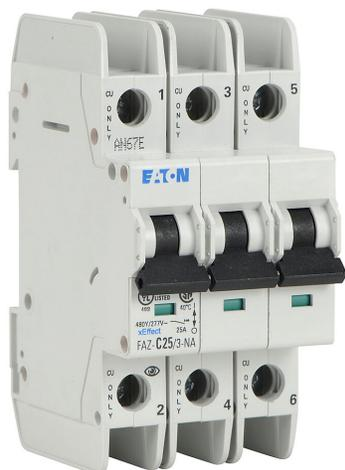
Eaton miniature circuit breaker, current-limiting, 25A, 480Y / 277 VAC / 96 VDC, 3-pole, C curve, thermal magnetic, 14kA @ 480Y/277 VAC interrupting rating, 35mm DIN rail mount.
