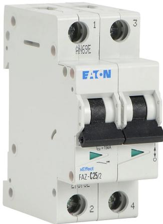
Eaton miniature supplementary protector, 25A, 480Y / 277 VAC / 96 VDC, 2-pole, C curve, thermal magnetic, 10kA @ 480Y/277 VAC interrupting rating, 35mm DIN rail mount.
