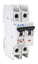
Eaton miniature circuit breaker, current-limiting, 25A, 240 VAC / 96 VDC, 2-pole, C curve, thermal magnetic, 14kA @ 240 VAC interrupting rating, 35mm DIN rail mount.
