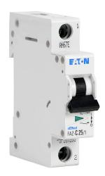
Eaton miniature supplementary protector, 25A, 277 VAC / 48 VDC, 1-pole, C curve, thermal magnetic, 10kA @ 277 VAC interrupting rating, 35mm DIN rail mount.
