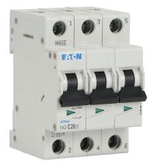
Eaton miniature supplementary protector, 20A, 480Y / 277 VAC / 96 VDC, 3-pole, C curve, thermal magnetic, 10kA @ 480Y/277 VAC interrupting rating, 35mm DIN rail mount.
