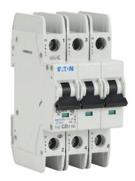
Eaton miniature circuit breaker, current-limiting, 20A, 480Y / 277 VAC / 96 VDC, 3-pole, C curve, thermal magnetic, 14kA @ 480Y/277 VAC interrupting rating, 35mm DIN rail mount.
