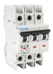
Eaton miniature circuit breaker, current-limiting, 20A, 240 VAC / 96 VDC, 3-pole, C curve, thermal magnetic, 14kA @ 240 VAC interrupting rating, 35mm DIN rail mount.
