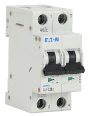
Eaton miniature supplementary protector, 20A, 480Y / 277 VAC / 96 VDC, 2-pole, C curve, thermal magnetic, 10kA @ 480Y/277 VAC interrupting rating, 35mm DIN rail mount.
