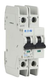
Eaton miniature circuit breaker, current-limiting, 20A, 480Y / 277 VAC / 96 VDC, 2-pole, C curve, thermal magnetic, 14kA @ 480Y/277 VAC interrupting rating, 35mm DIN rail mount.
