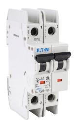
Eaton miniature circuit breaker, current-limiting, 20A, 240 VAC / 96 VDC, 2-pole, C curve, thermal magnetic, 14kA @ 240 VAC interrupting rating, 35mm DIN rail mount.
