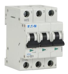
Eaton miniature supplementary protector, 2A, 480Y / 277 VAC / 96 VDC, 3-pole, C curve, thermal magnetic, 10kA @ 480Y/277 VAC interrupting rating, 35mm DIN rail mount.
